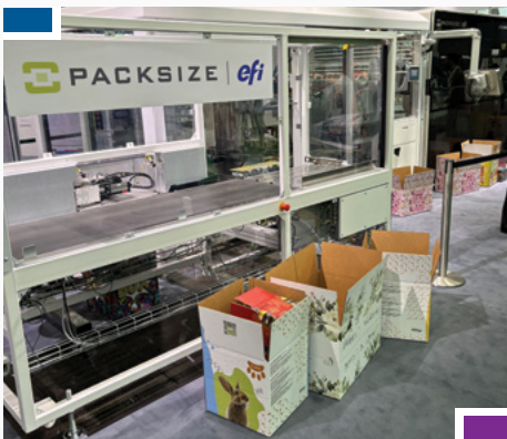
The Packsize EFI X5 Nozomi, featured at drupa 2024, is a fully automated on-demand packaging system
