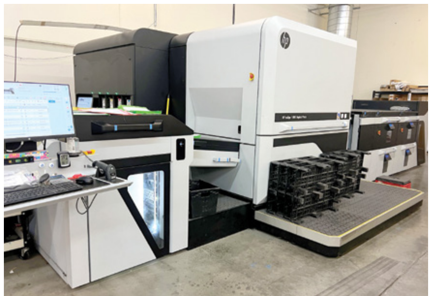
(Top right) Book printed for Jackson Suites by Corefact. (Right) HP Indigo 100k Digital Press. The world's most productive B2 digital solution (compared to alternative B2 digital commercial solutions as of November, 2019), with true digital non-stop print capabilities, at 6,000 sheets per hour.
